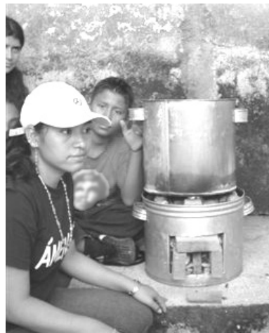
Wood cookstove workshop. Twig-sized wood goes in small hole at the base.
